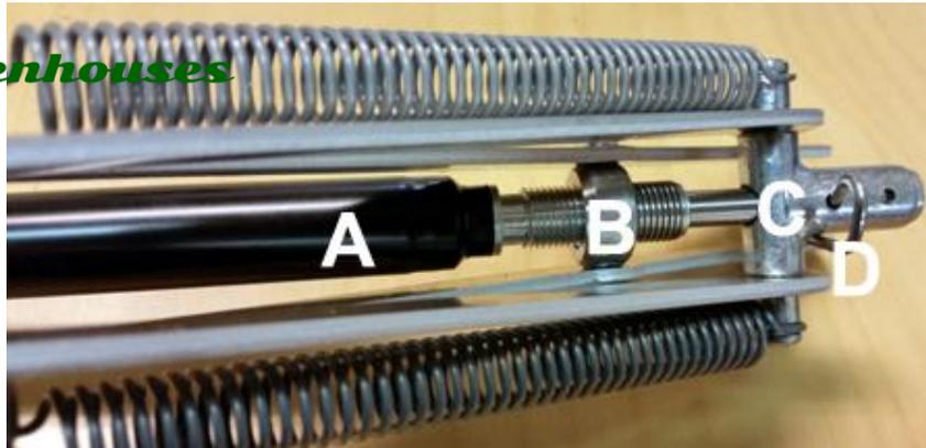
4. Insert the Black Rod Cylinder (A) through the round cylinder housing (B) and through the top hole of the Clutch T (C).
