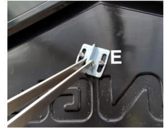
10. Attach the Vent Bracket (E) to the black vent, using **two Oversized Rivets**. Mark the vent where the holes go. Drill from the inside. Riveting from the outside of the vent door will give a clean finished rivet look. Hold the Vent Bracket (E) tight against the door during this procedure. Assistance comes in handy here.
